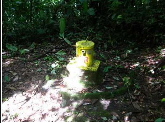
Photo 157: I-5 I-19 I-17 Piezometer in a fauna relocation area in ICE's land
