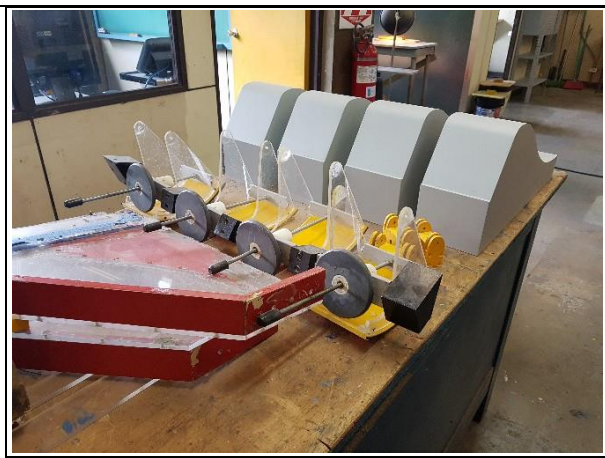
Photo 49: Dismantled parts of the model of the gated spillway at ICE offices in San Jose (I-5)
